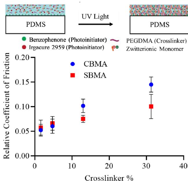
**Figure 1.** A schematic of the new method for hydrogel formation. Data for the coefficient of friction relative to uncoated biomaterial for different crosslink densities.
